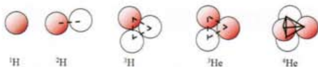
Figure 1: Schematic illustration of the nuclear bond changes during the fusion of two deuterons to form an alpha particle
